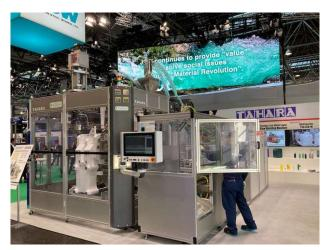
In addition to the machine, we displayed 20L jerry can and 500ml bottles made of the resin sourced from maritime industry waste. Multilayer molding is suitable for recycled resin. By molding in 3layers, recycled resin can be put between virgin layers. It prevents from leaking recycled resin scent, spoiling the appearance and dissolving to the contents.
